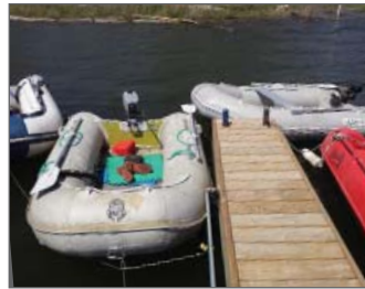
Tethers too long and in the wrong location. Dinghies are interfering with the workboat and each other.
